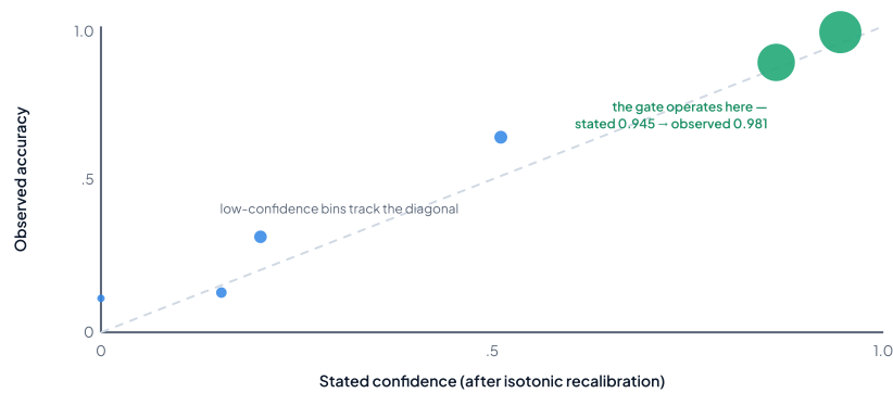
Fig. 3 — Reliability diagram, diagnosis confidence (held-out test set: 376 charts, 1,496 scored diagnosis codes in bins). Each dot is a confidence bin (area \propto bin size); the diagonal is perfect calibration. After isotonic recalibration (fit on the development split, applied unchanged), expected calibration error is 0.037 on the test set (0.026 across all charts) — and the top bin, where the auto-finalize gate operates, runs slightly conservative : codes stated at 0.945 confidence were right 98.1% of the time.
